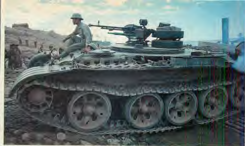
ABOVE: Vietnamese 9th Division Armored Recovery Vehicle (ARV). Base for ARV is modified Russian T-54 or Chinese Type 59. In two-part cupola either the Vietnamese or Chinese have mounted 7.62mm machine gun to complement 12.7mm DShK anti-aircraft gun (note anti-aircraft sight on the 12.7mm). Vehicle also has mounted jib crane, probably used to tow stuck vehicles.
